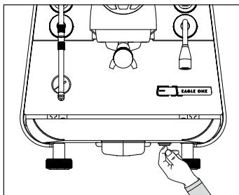
Switch ON the machine by pressing the switching button situated on the bottom right side.
