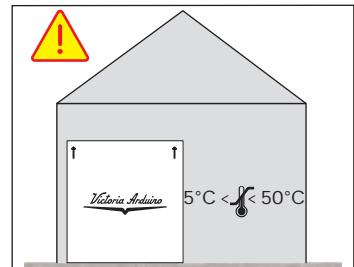
The package containing the machine must be stored away from atmospheric agents. Before performing the following operations, make certain that the load is in stable and will not fall when the straps are cut.
